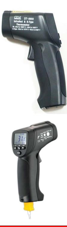
HT-8855 CE certified digital IR Laser thermometer. This top-of-the-line compact device features 30:1 D/S ratio, K type temperature probe, analog output and wireless USB interface. The IR thermometer can be used to measure surface temperature quickly and conveniently, while the K type temperature probe can be used to measure air / vapor temperature accurately.
